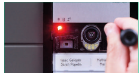
9. THROUGH the dedicated selector, enter the programming mode (you know you are in the programming mode because the dedicated LED comes on) and THROUGH dip switch, select the first address to be assigned to the first button
