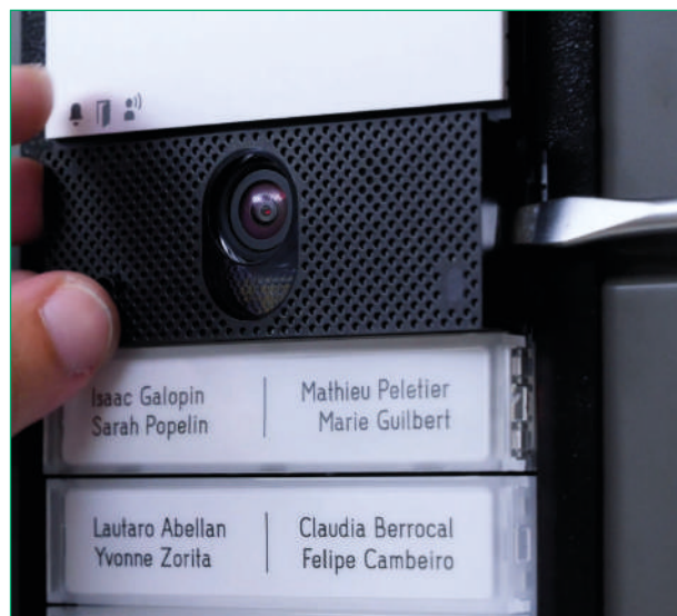
8. REMOVE the front panel to access the various programming modes/settings
