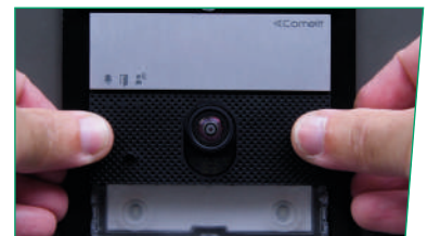
7. ATTACH the audio/video module, button modules and nameplates
