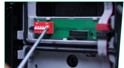
6. CONFIGURE the type of button that will be used (single/double) and an address in the button module
