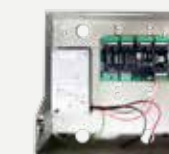
Controller: 512 - DC, enclosure, 3A PSU
